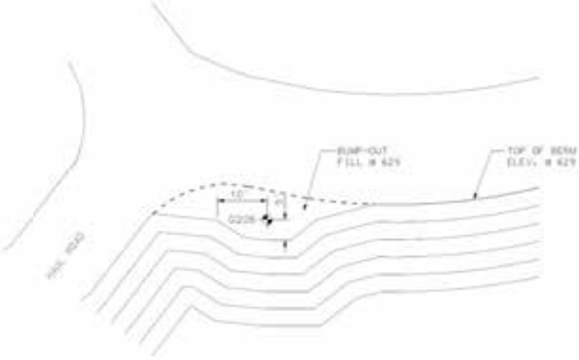
2 05 MONITORING WELL BUMP-OUT AT HAUL ROAD
