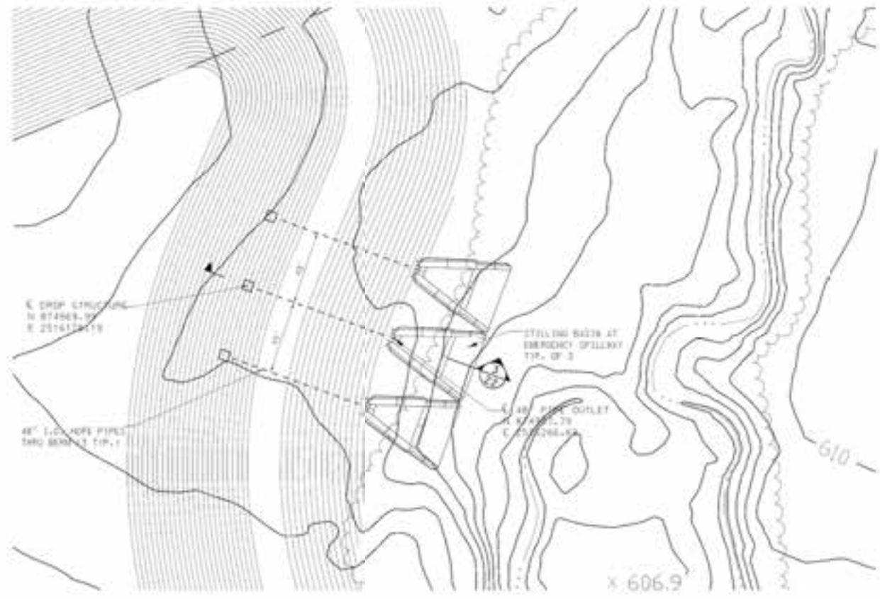
1 STILLING BASIN PLAN AT EMERGENCY SPILLWAY NTS
